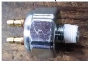
trip to the Rubber Connection for a new switch at \$14.25 with Club discount. After returning home the new switch was loaded with a couple of turns with Teflon tape on the thread and screwed into the block bolt. This time I did not use as much force tightening the switch but the large ring spanner made the job easy. I used a 1" inch AF ring spanner on the switch, as it is hexagonal in shape, and I held the connector block bolt from turning, with a
