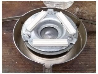
then allowed the end connector to protrude below the shroud which the spring could contact. The spring then contacted the locating ferrule which sat in the steering column completing the electrical circuit which caused the HORN to start blaring.
