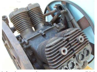
was one of seven experimental X-8 engines—and 58 experimental engines total—once left to sit in a sugar beet mill building on the Greenfield Village campus. While records for the experimental engines were incomplete, the seven X-8 engines include both air-cooled and water-cooled L-heads as well as at least one aluminum air-cooled overhead-camshaft version.
