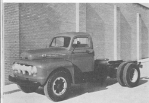
This F-7 Big Job will be fitted with a "fifth wheel" for tractor duty.
